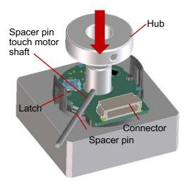
Press down on the hub gently while tightening the set screw with the hex wrench. The recommended torque to tighten the set screw is 0.10 Nm to 0.13 Nm (0.9 in.lb to 1.15 in.lb). A threadlocker can be applied to set the screw threads to prevent the screw from unthreading during operation.
